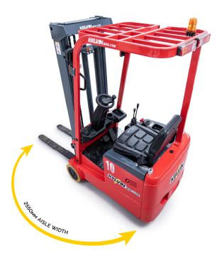
**Low closed height** The Kelvin Mini has a closed height of 1965mm
